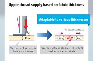
By automatically analyzing the stitch type and fabric thickness, i-TM supplies the optimal amount of thread for the best embtroidery finish at all times.
