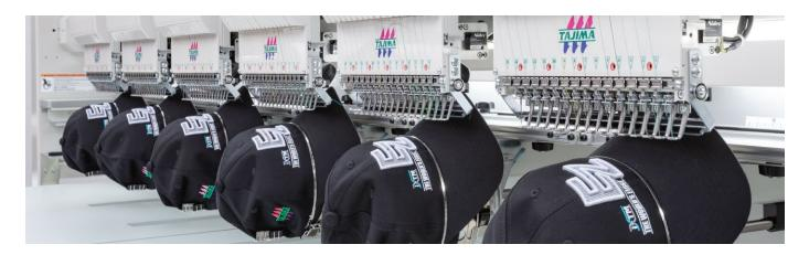
Reinforcement of the cap frame support structure has contributed to stabilization of the embroidery finish, by dramatically increasing the maximum rotation speed up to 1,000 rpm.
