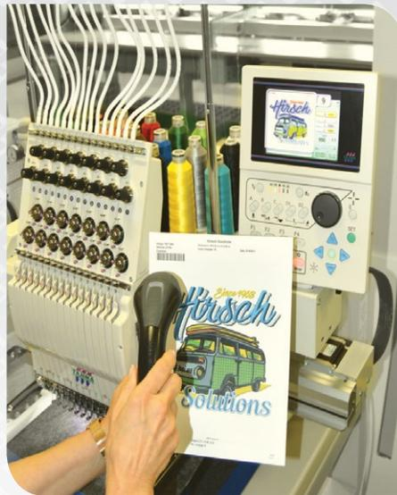
Barcode scanners can instantly load embroidery designs into the machine memory with a single click and will also automatically program the design color sequence based on the needles selected in the design.
