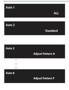
Perform automatic adjustment for all patterns (A to F) using the color sensor.
