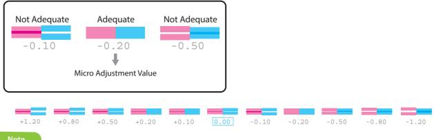
Once an appropriate micro adjustment value has been saved, the value will be the baseline value from the next time to be printed in the center of the pattern.
