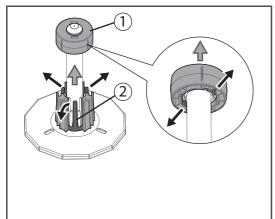
(If you are using 2-inch core roll media) Remove the 3-inch adapters from the media flange.
