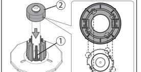
(When replacing 2-inch core roll media with 3-inch core roll media) Attach the 3-inch adapters to the media flange.
