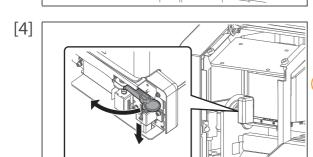
Press the cutter cap lightly, turn Cutter holder in the direction as illustrated below.
