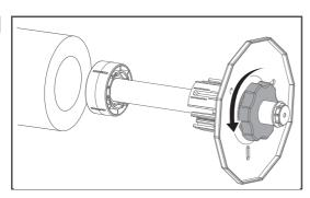
Push the media flange (×2) into the both ends of the media core.
