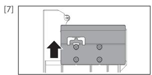
Do the same for the left media holder to slide up the roller shaft guide plate as far as it will go and tighten the screws.
