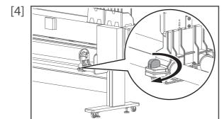
Twist the knob bolt on the right side of the media holder clockwise to tighten.
