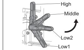
Use the head height adjustment lever (orange) to change the head height.
