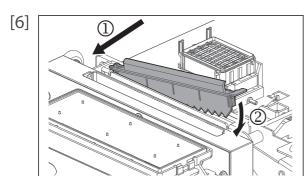
Attach an appropriate cleaning wiper to the wiper slot.
