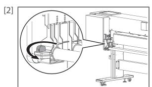
Twist the knob bolt on the left side of the media holder anticlockwise to loosen.
