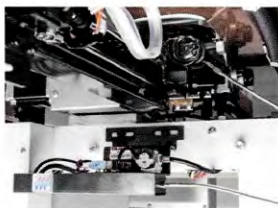
ABC : Auto Bobbin Checker Device to detect the remaining amount of bobbin thread
