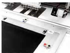
Bar Code Reader To confirm design data and materials in order to avoid human error.
