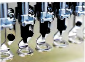
Knife to make holes There are 3 types of perforator needles (1.0mm, 1.5mm, and 2.0mm) according to hole size.
