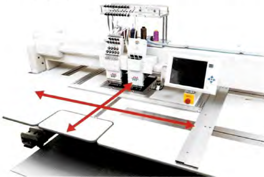
Wider Sewing Area due to Bridge Structure
