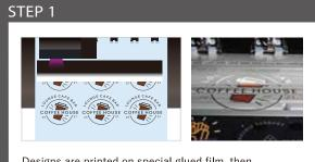
Designs are printed on special glued film, then application sheet is pasted on the film autimatically.
